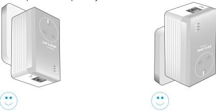
All powerline adapters and extenders should be on the same electrical circuit.
